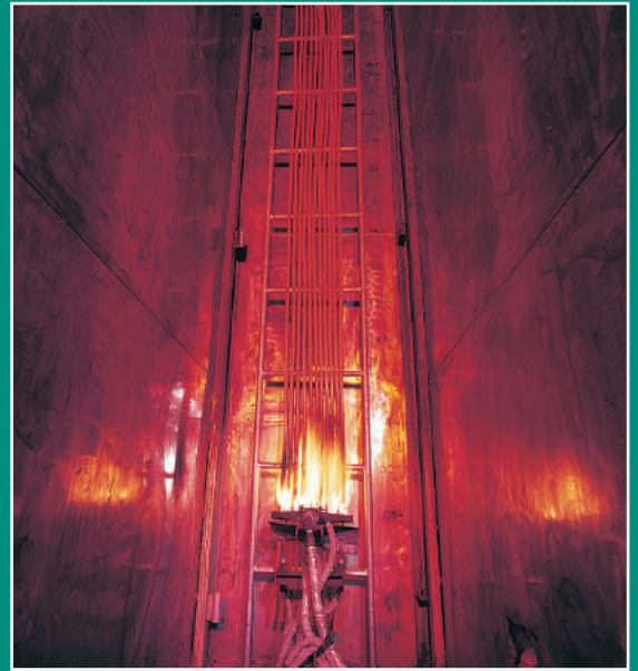
Flame Retardant Test Equipment - IEC 60332-3
