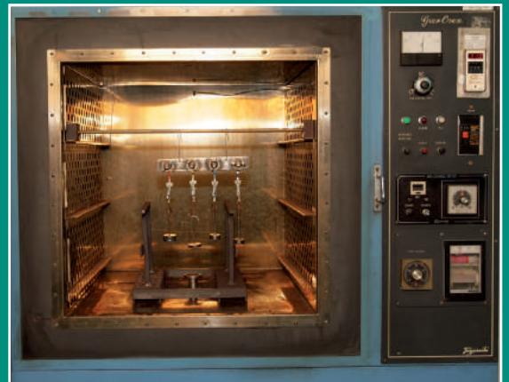
XLPE Hot Set Test Equipment - Oven
