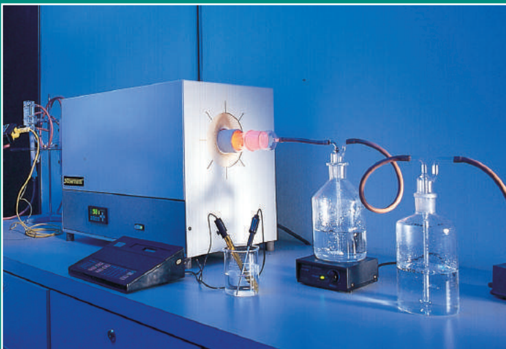
Halogen Content & Corrosivity Tests Equipment - IEC 60754-1 & IEC 60754-2
