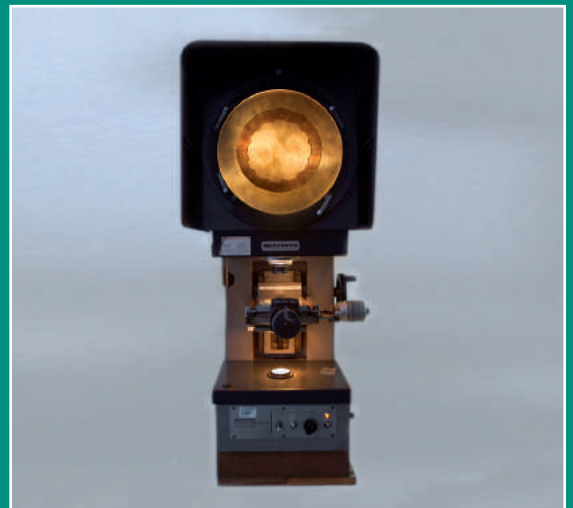
Wall Thickness Measuring Equipment - Profile Projector
